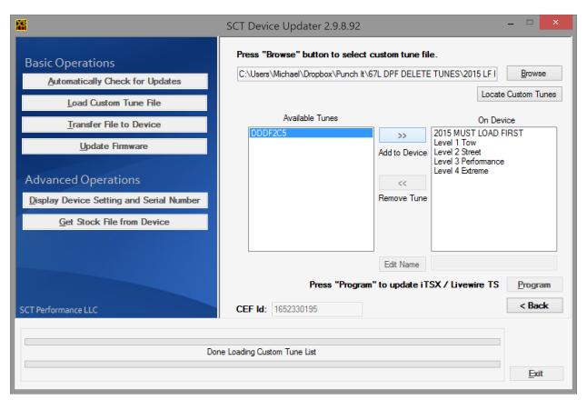
STEP 5- Plug tuner into vehicle, select Program Vehicle, (DO NOT SELECT Pre Loaded Tunes at top)
